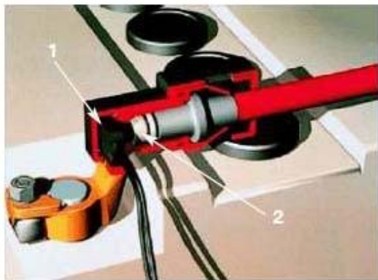
Fig. 27: Seat Belt Pre-Tensioner
