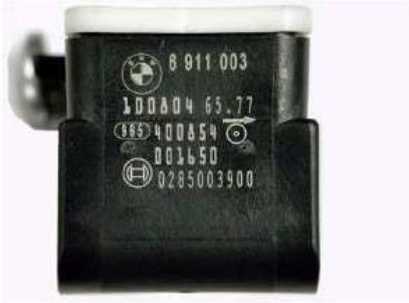
Fig. 5: B-Pillar Satellite (1 Of 2)
