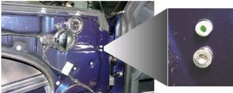
Door Pressure Sensor Mounting
