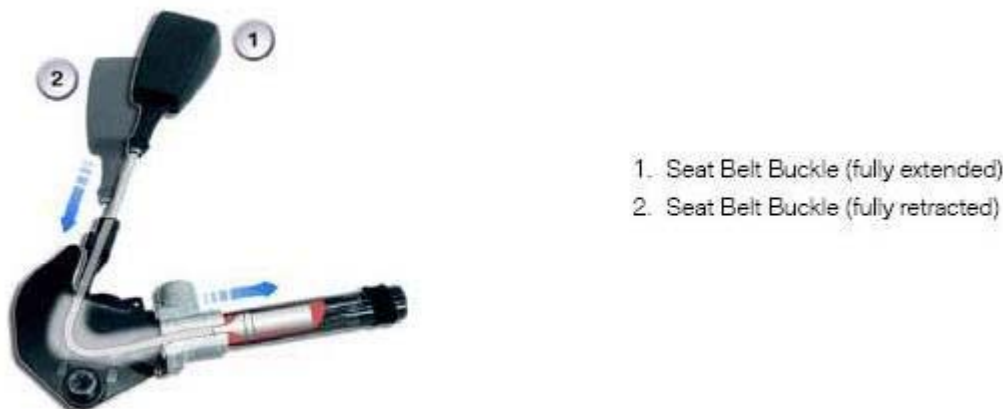
Fig. 26: Seat Belt Pre-Tensioners
