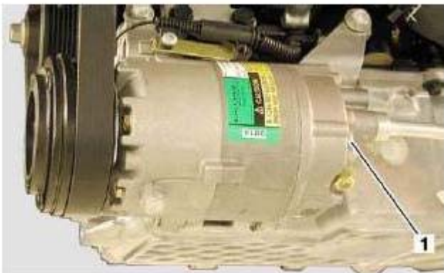
Compressor Mounted on Engine
