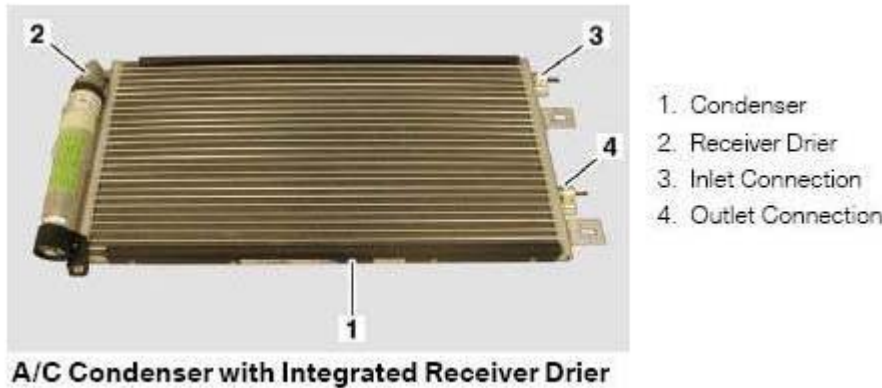
Fig. 9: A/C Condenser With Integrated Receiver Drier Courtesy of BMW OF NORTH AMERICA, INC.
