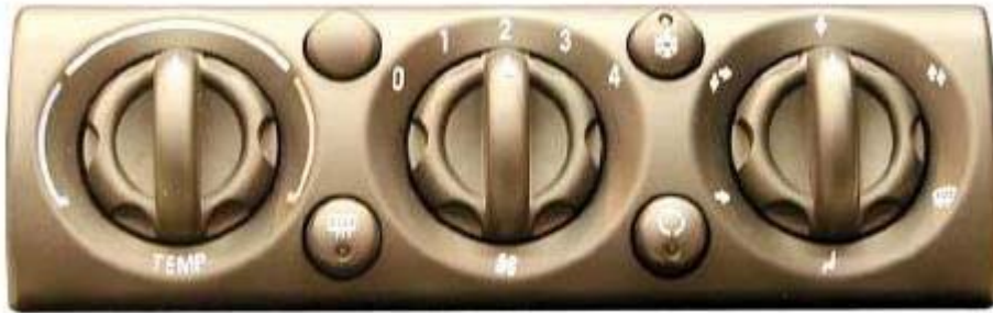
Fig. 28: Switch Panel (IHKS)
