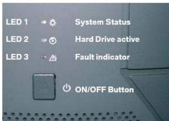
Fig. 6: System Indicators And ON/OFF Button Courtesy of BMW OF NORTH AMERICA, INC.
