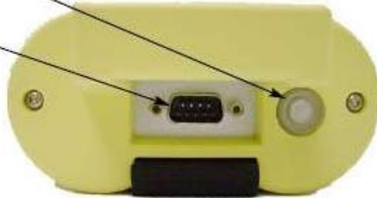
Fig. 11: Signal Recorder Button And Serial Interface Connection Courtesy of BMW OF NORTH AMERICA, INC.
