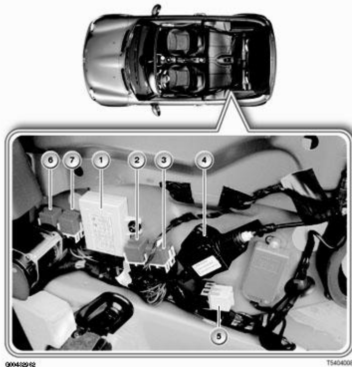
Fig. 2: Locating Convertible Top Module And Relays Courtesy of BMW OF NORTH AMERICA, INC.
