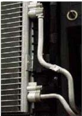
A/C Lines at Condenser
