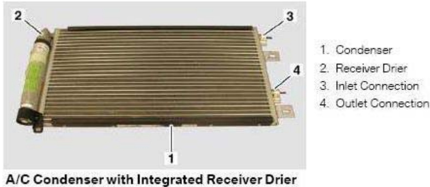
Fig. 9: A/C Condenser With Integrated Receiver/Drier Courtesy of BMW OF NORTH AMERICA, INC.
