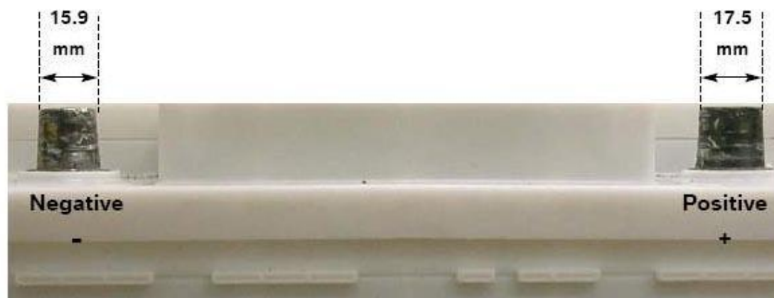
Fig. 5: Battery Positive And Negative Terminals Courtesy of BMW OF NORTH AMERICA, INC.
