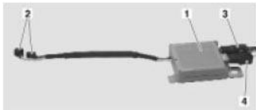
Aerial Amplifier Unit 44-08-102 Located in the Tailgate on the left side
